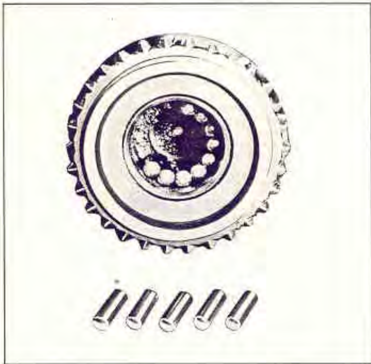
Fig. 78-25 Loading Bearings Into Main Drive Gear
